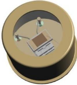
1. **CLEANING:** Clean the package window with a 50/50 mixture of isopropyl alcohol and water. Either rinse package gently, or use light strokes with a cotton tipped applicator. Care must be taken to avoid using excessive pressure on the window as you may destroy the hermetic seal. Do not use acetone or halogenated solvents. **NEVER** use an **ULTRASONIC CLEANER** to clean detectors or detector assemblies.
